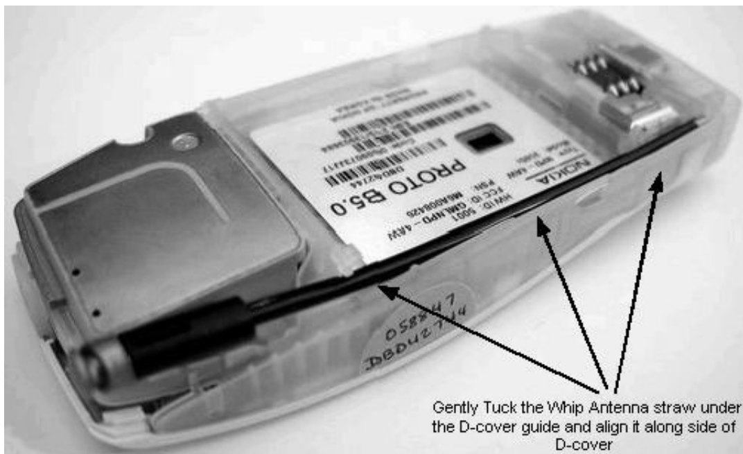
Figure 5: Properly installed whip antenna
